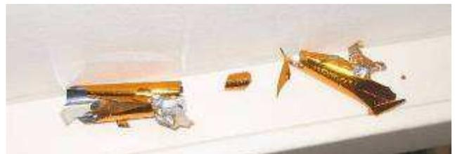
Test samples with new coatings, new protective lacquers, and combinations thereof were obtained (see Figure 49) for testing their ability to withstand high thermal loads due to the high radiative flux impinging on them. The samples were tested by placing them close to the Xe arc lamps (see Figure 50)
