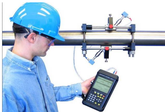
Ultrasonic flowmeters can be installed out of the pipe, allowing on site inspection at different location with the same instrument
