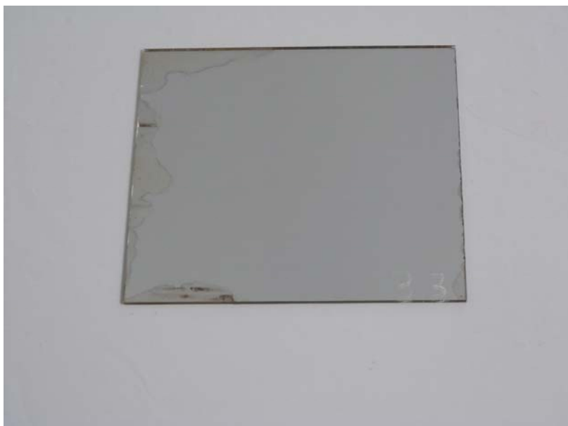
Figure 14 Sample 3 edges degradation example, after damp heat test
