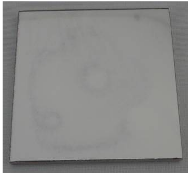
Figure 12 Degradation stains due to a glue chemical reaction (sample 5), after humidity test
