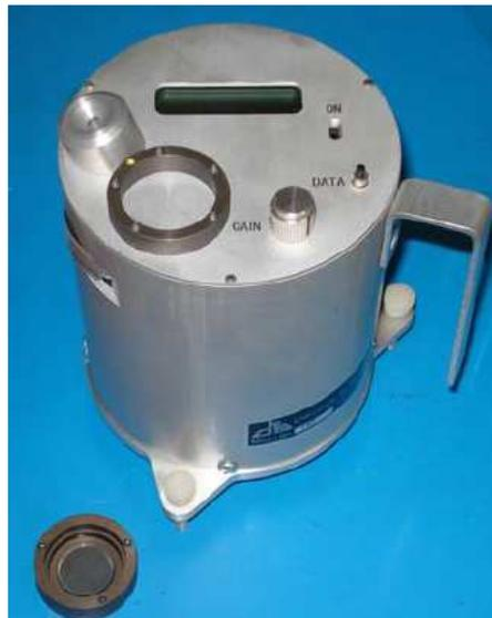
Figure 12: Portable specular reflectometer 15R by Devices and Services [3].
