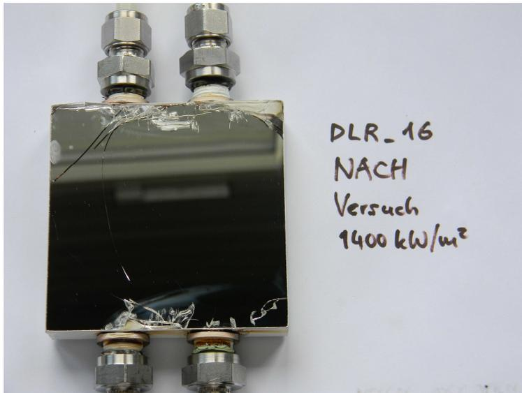
Figure 14: Sample DLR\_16 after irradiation with  $1400 \text{ kW/m}^2$  showing mechanical cracks (part of which were already visible before the thermal tests, see Fig. 4), but no traces of mirror melting.
