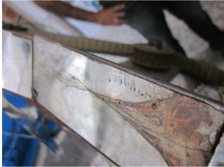
Figure 5 Glass cover losses and silver corrosion.
