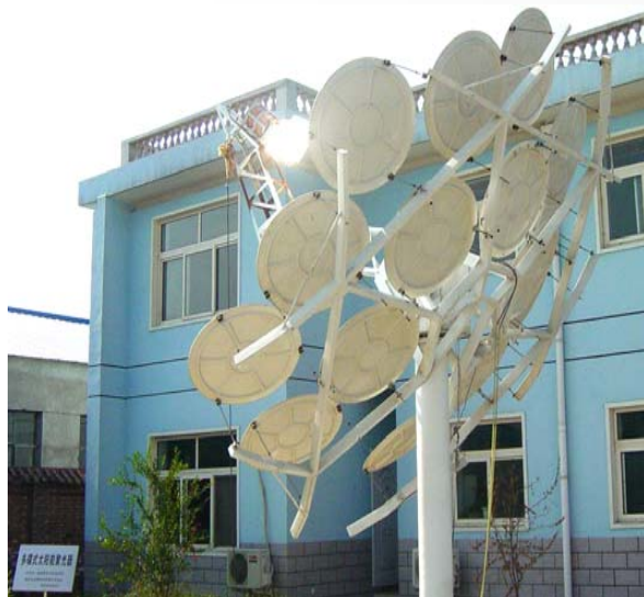
1KWe dish Stirling system by IEECAS and Himin Solar, 2005
